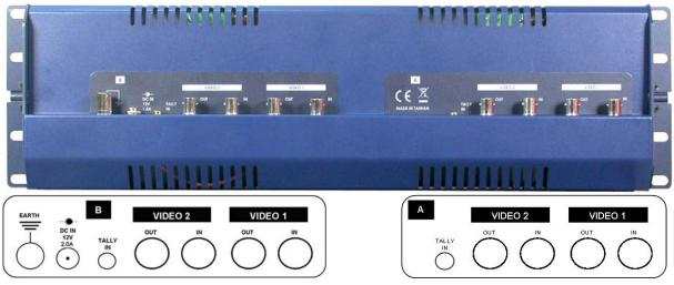
The earth terminal can be used with other equipment that has the same feature. Connect all items together to ensure that they are grounded.
